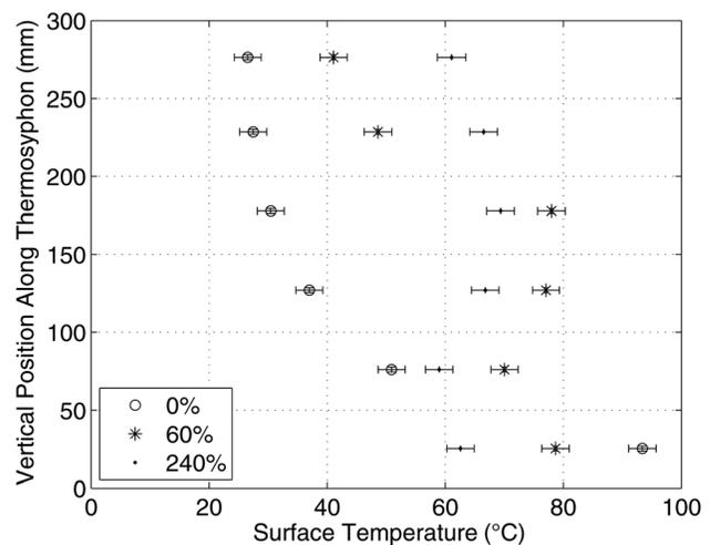
Fig. 3 The surface temperature as measured by thermocouples placed along the length of the condenser section of the thermosyphon for the 0%, 60%, and 240% fill volumes when the evaporator temperature is 157 °C
