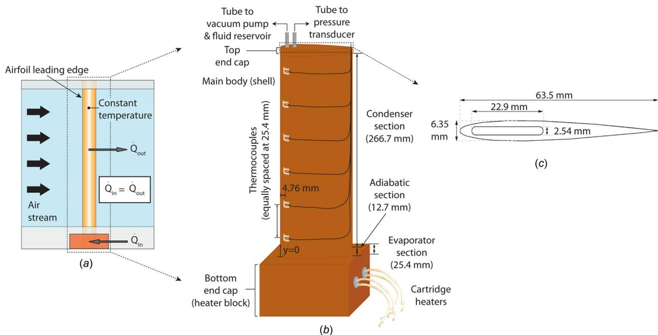
Fig. 1 (a) Schematic of the steady state experimental setup in the wind tunnel test section, (b) side view of the thermosyphon assembly with thermocouples attached, and (c) thermosyphon cross section with labeled dimensions
