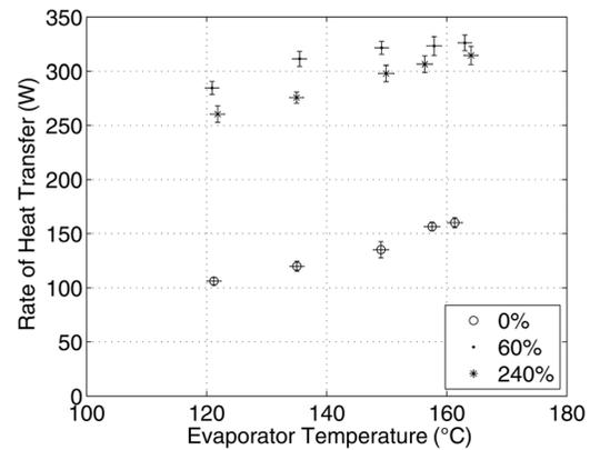
Fig. 2 The rate of heat transfer as a function of evaporator temperature for the 0%, 60%, and 240% fill volumes
